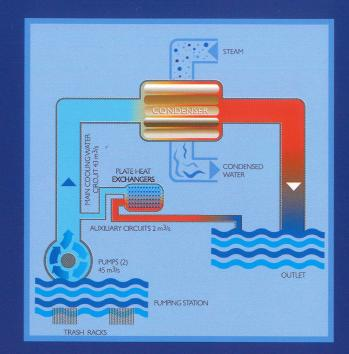
Biofouling control methods are based on the use of two different classes of antimicrobial or biocidal products:
